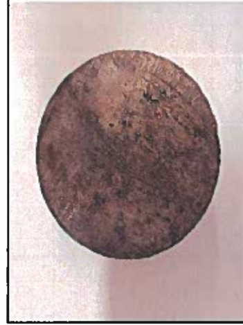
Photos 7 & 8: BH18-107 Sa R2 Cerchar before and after testing
